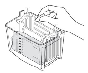
8. Put on the lid, plug the cables into the power supply. and run the blot. Refer to Section 3 for run times and voltage settings with various buffers.
