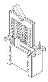
6. Add the frozen blue cooling unit. Place in tank and fill to the "blotting" mark on the tank.
