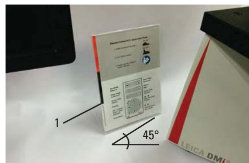
Fig. 22 Mounting camera IR reflection shield 1 IR reflection shield
