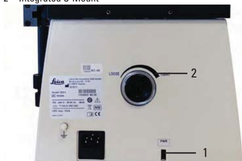
Fig. 19 Rear view of the stand 1 Camera USB power supply port (PWR port) 2 Integrated C-Mount
