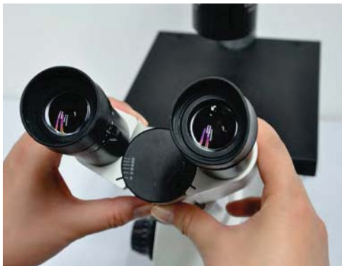
Fig. 24 Adjusting the eyepieces
