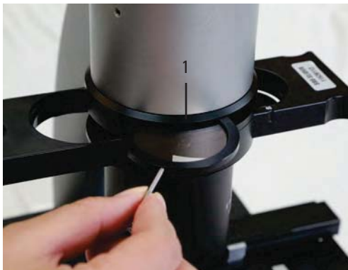
Fig. 15 Insert of transmitted light filter 1 Transmitted light filter slot
