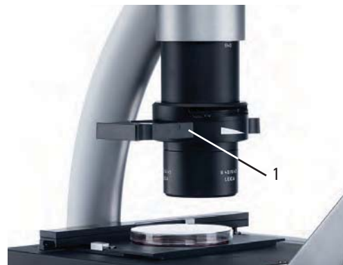
Fig. 18 Inserting the phase contrast slider 1 Phase contrast slider
